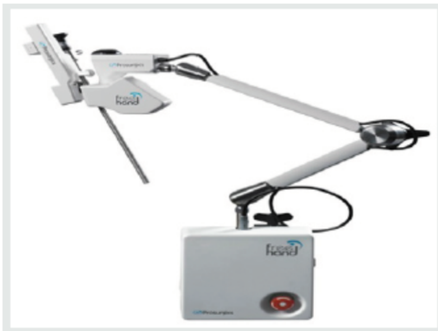
Figure 1: FreeHand® Camera holder with laparoscopic lens attached.
